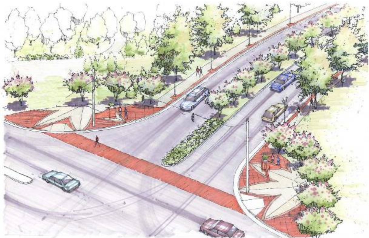
Typical Intersection demonstrating crosswalk patterns, ramps, downtown streetlights, and median potential for Williamson Road
